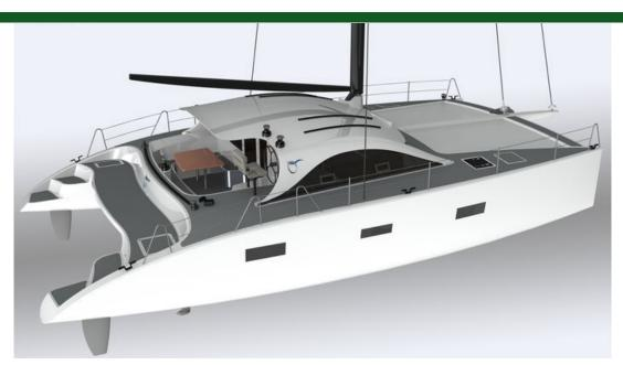
Modern Type Propulsion Sail Hull Catamaran 14.0m (46') Length Beam 7.6m (25') Draft 1.1m (4') **Hull Material** Composite 2 / Yanmar / Engine
