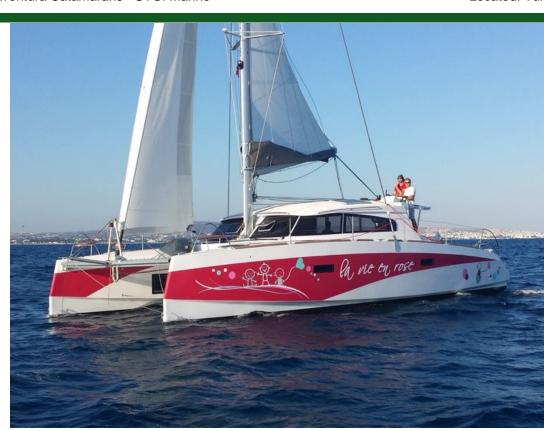
Type Modern Propulsion Sail Hull Catamaran Length 13.2m (44') Beam 7.0m (23') Draft 1.3m (5') **Fiberglass Hull Material Engine** 2 / Nanni / **Engine HP** 37.5
