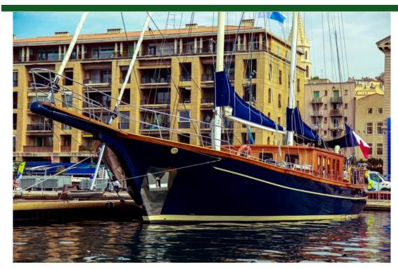
种类经典游艇类型帆船船身类型单体船载客量25.8m (85 ' )船宽6.5m (22')吃水2.9m (10')船身材料钢
