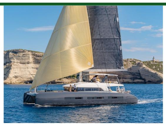
种类现代游艇类型帆船船身类型双体船载客量23.7m (78 ' )船宽11.0m (37')吃水1.9m (7')船身材料玻璃钢
