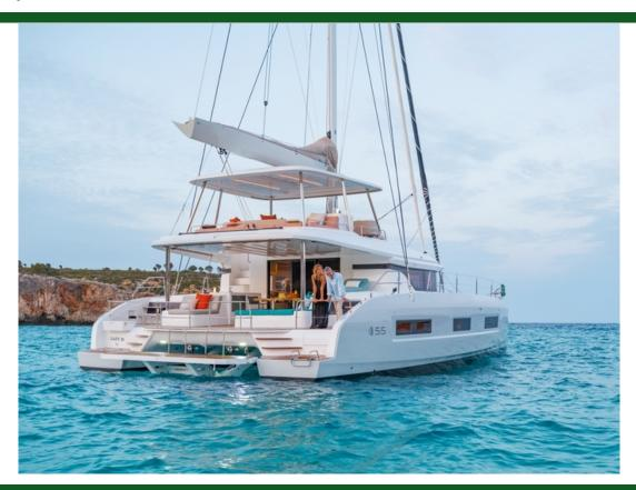
种类现代游艇类型帆船船身类型双体船载客量16.5m (55 ')船宽9.0m (30')吃水1.5m (5')船身材料玻璃钢
