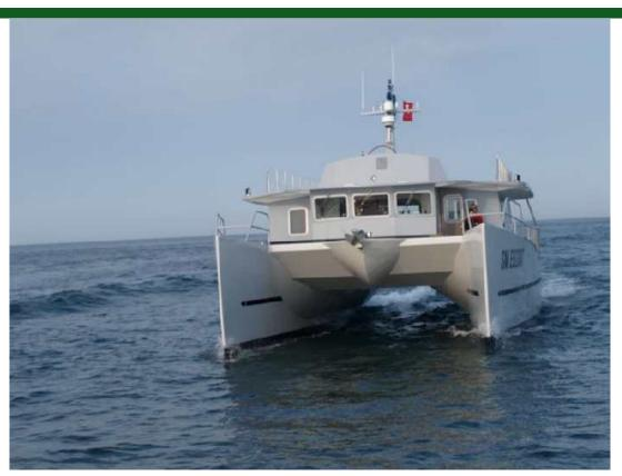
**Project** Type Propulsion Power Hull Catamaran Length 20.0m (66') Beam 8.7m (29') Draft 1.5m (5') **Hull Material** Wood **Engine** 2 / Iveco / **Engine HP** 270
