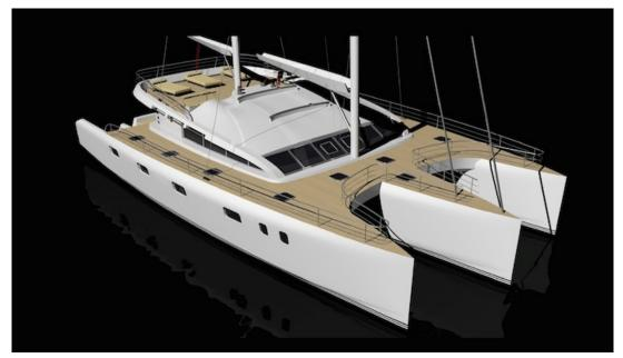
Project Type Sail Propulsion Hull Trimaran Length 24.0m (79') Beam 11.9m (40') Draft 1.5m (5')
