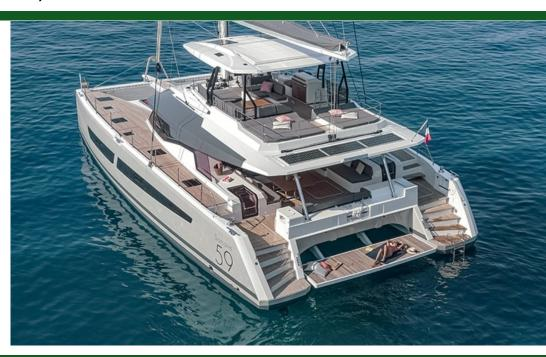
Type Modern Propulsion Sail Hull Catamaran 18.8m (62') Length Beam 9.5m (32') Draft 1.6m (6') **Hull Material Fiberglass** Engine 2 / Volvo / Engine HP 110
