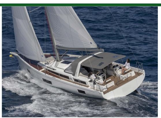
Type Modern Propulsion Sail Hull Mono 17.1m (57') Length Beam 5.0m (17') 2.5m (9') Draft **Hull Material Fiberglass** Engine 1 / Yanmar /
