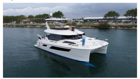
Type Modern Propulsion Power Hull Catamaran Length 13.4m (44') Beam 6.5m (22') Draft 1.0m (4') **Hull Material Fiberglass**
