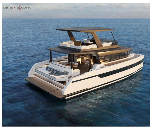
Type Modern Propulsion Power Hull Catamaran Length 15.0m (50') Beam 7.5m (25') Draft 0.9m (3') **Hull Material Fiberglass** Engine 2 / Torqeedo /
