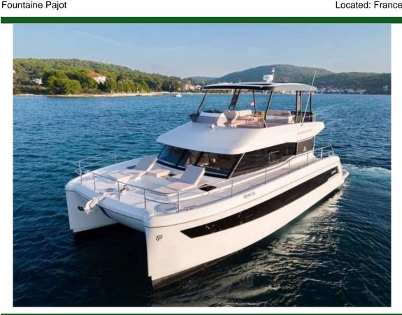
Modern Type Propulsion Power Catamaran Hull Length 14.0m (46') Beam 6.0m (20') 1.3m (5') Draft **Hull Material Fiberglass**
