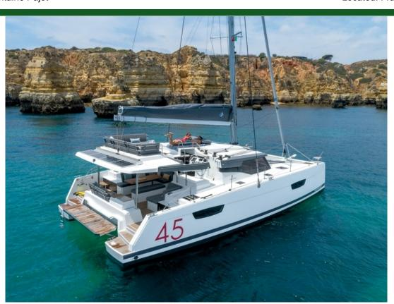
Modern Type Propulsion Sail Catamaran Hull Length 13.5m (45') Beam 7.5m (25') 1.2m (4') Draft **Hull Material** Fiberglass 2 / Nanni /
