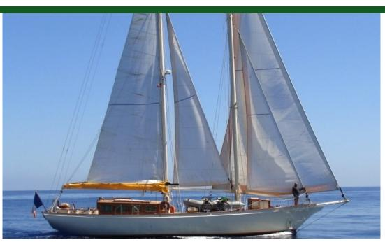
Classic Type Propulsion Sail Hull Mono Length 17.6m (58') Beam 5.2m (18') 2.4m (8') Draft Aluminium **Hull Material** 1 / Nanni / 6660 Engine
