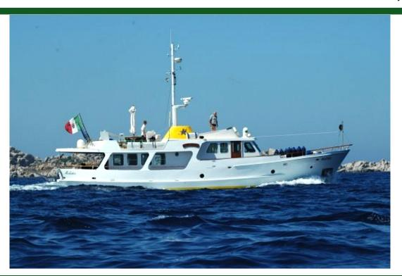
Type Classic Propulsion Power Hull yacht 19.0m (63') Length Beam 5.2m (18') Draft 2.0m (7') **Hull Material** Steel Engine 2 / Cumins /
